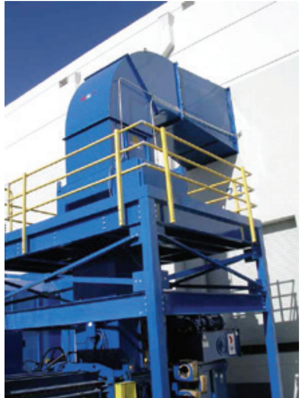
A BloApCo top feed shredder with a four side work platform mounted over an inline horizontal baler. In this installation the shredder and baler are outside the building to maximize space in the plant.
